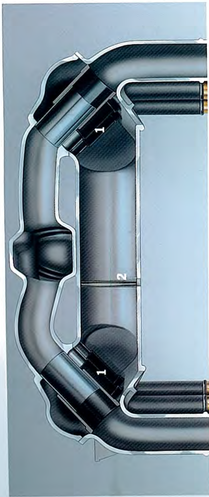
Varioram. Single-chamber induction system: Shift-tube extension (1) and resonance flaps (2) shut. Optimization of torque at low and medium revolutions.
